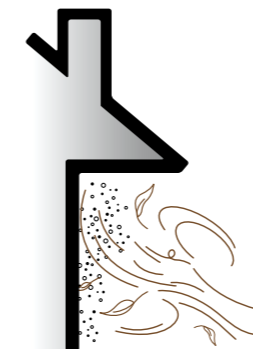
Dust carried by the wind is also a source of corrosion.
