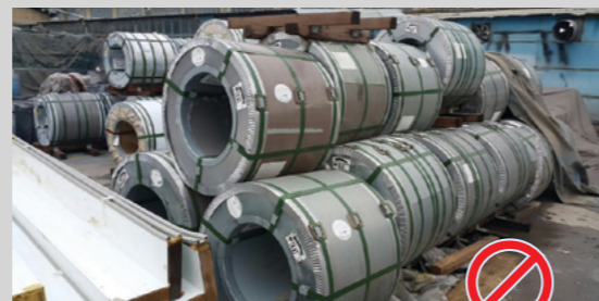
▲ Incorrect outdoor storage (cover not used)
