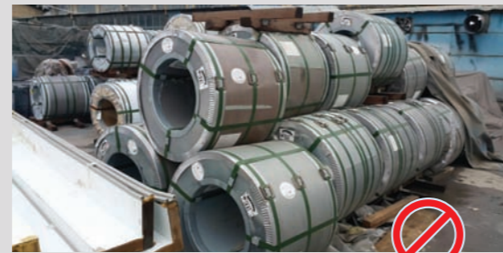
▲ Incorrect outdoor storage (cover not used)
