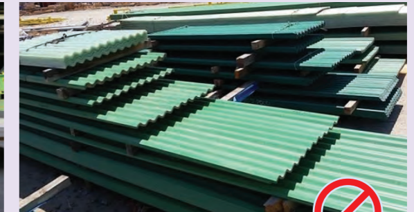
▲ An example of non-use of a cover and poor drainage
