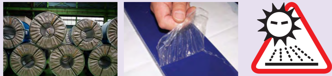
▲ A method of stacking products with a protective film (Avoid two-tier stacking)
