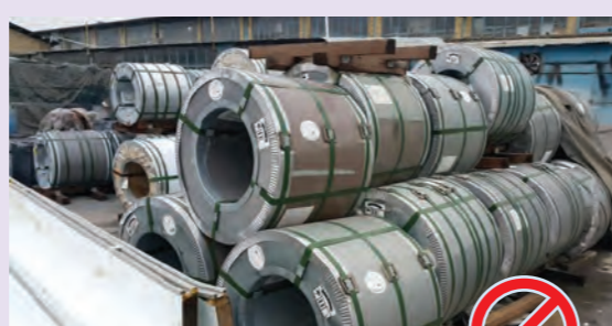
▲ An example of incorrect outdoor storage (A cover is not used)
